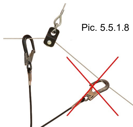
Pic. 5.5.1.8: Only hook into horizontal parts of the Savekingline® with a horizontal deviation < 3^\circ
